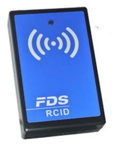
The competitor ID remote control RCID automates your training timing requirements by allowing your competitors to self-identify themselves to our TBox and iOS app before they leave the start. A 125khz RFID antenna mounted at the start, detects our RFID badges or wristband worn by the competitor.
